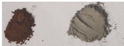
Figure IV - 53: LFO powders – left side (rust brown colored) is LFO exposed for 5 days in ambient laboratory air, and right side powder (gray colored) is the LFO stored in a vial in the dry room for 5 days.
