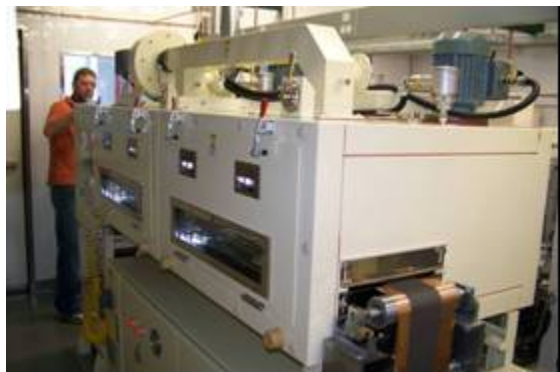
Figure IV - 154: "Reverse comma" coater with dual drying zones and intermittent coating capabilities.
