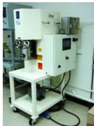
Figure IV - 156: High energy/shear planetary mixer from Ross with a 2 liter chamber capacity.
