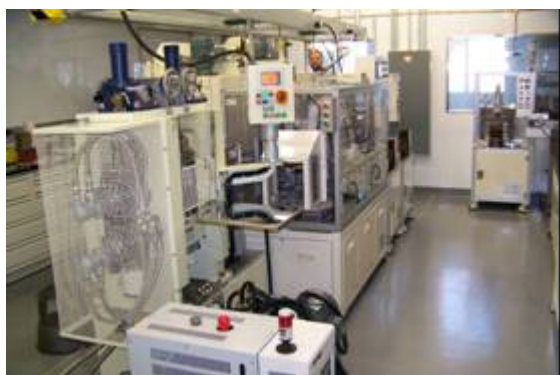
Figure IV - 155: Hot roll press capable of 1.5 tons/cm force and 120°C roll temperature.
